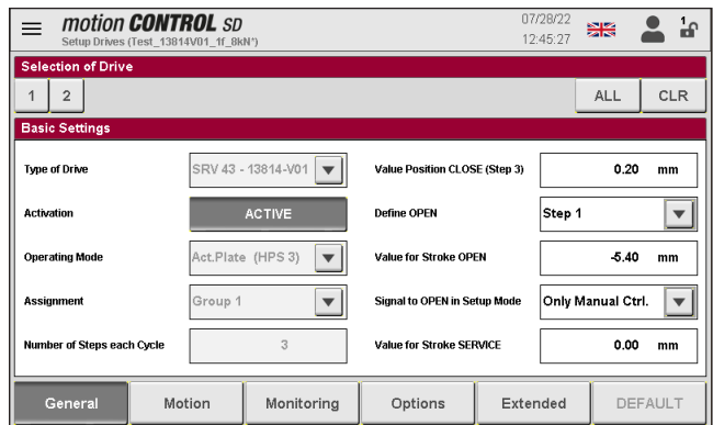
Picture 21: View „Configuration of drives – Basic Settings“ / motion CONTROL SD for synchronous plate systems“
